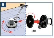
Scrub the floor using clean black or high-performance pads. Flip or change pads as needed.
